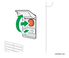
The main power indicator on the right side of the control panel turns off. The main power turns off automatically after the machine has shut down properly.
