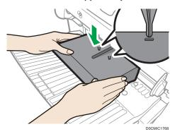
Attach the Z-fold support tray by inserting the two protrusions on its underside into the holes on the finisher shift tray.
