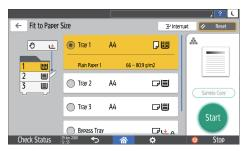
When the orientations of the original and paper in the paper tray do not match, the machine rotates the copied image automatically. To reduce an original of A3 (11 × 17) size to A4 (8 $^{1}/_{2}$  × 11) size, for example, you can select either A4 (8 $^{1}/_{2}$  × 11) $\square$  or A4 (8 $^{1}/_{2}$  × 11) $\square$ .
