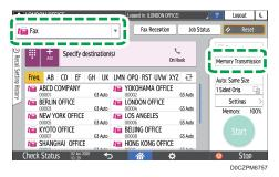
Press an item on the fax screen to select [Memory Transmission] if [Immed. Transmission] is selected.
