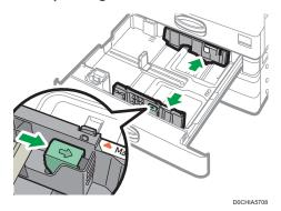
4. To load B4 JIS, A3, or 11 × 17 paper, pull the tray out completely and then change the positions of the two auxiliary side fences.
