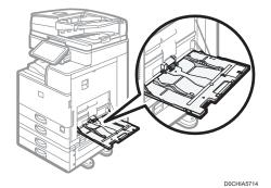
2. Load the paper with the print side down, and push it in lightly until you hear a beep.
