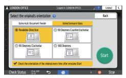
If the display of this screen is not necessary when you press [Start], clear the [Check the orientation of the original every time after pressing [Start]] check box.
