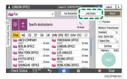
3. Press [Transmission Result], and select the transmission result to display.
