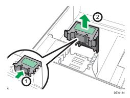
2. Put the auxiliary side fence into the groove for the paper size to use.
