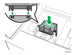
Change the position of the auxiliary side fence in the back in the same way.
