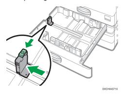
If the end fence is fixed with the stopper, rotate the fixing screw of the stopper 90 degrees counterclockwise with a coin or similar object and remove the stopper.
