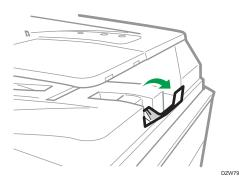
When using the ARDF to scan originals with a paper weight less than 42 g/m² (11 lb. Bond), move the slide tray on the original output tray to the left side. When the slide tray of the Auto Reversible Document Feeder (ARDF) is in the left, the amount of output paper will be low. After scanning a thin original, return the slide tray to the previous position.
