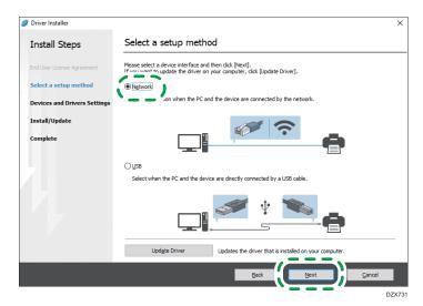
• The search detects devices connected to the network.
