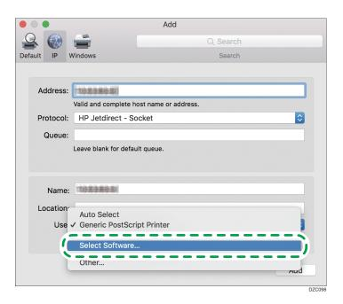
2. Select the machine on the "Printer Software" screen, and then click [OK].
