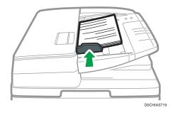
2. Place the aligned originals squarely face up in the one-pass duplex scanning ADF.
