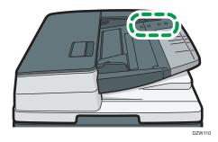
1. Place the originals flush against the rear paper guide and adjust the paper guides to the size of the originals.
