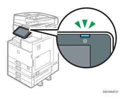
1. Open the cover of the main power switch on the front right side of the machine, and push the switch.
